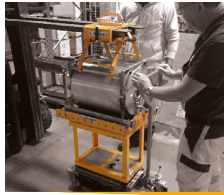
TABLE ELEVATRICE AVEC L'ACCESSOIRE DE LEVAGE POUR ONDULEUR
