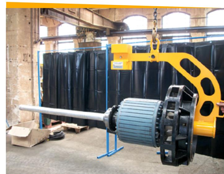
▶ CE DE LEVAGE ROTOR AVEC GUIDE DE MONTAGE CMU 0T500
